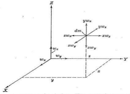
axes chosen to represent the airplane (Figure 10-2) are moving axes, the acceleration and rates of change of moment of momentum along and about the airplane axes must be referred back to the axes fixed in space.
