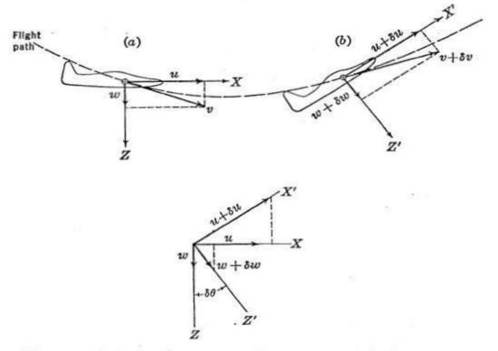
The rate of change of moment of momentum relative to fixed space can be developed in a similar way from Figure 10-6.
