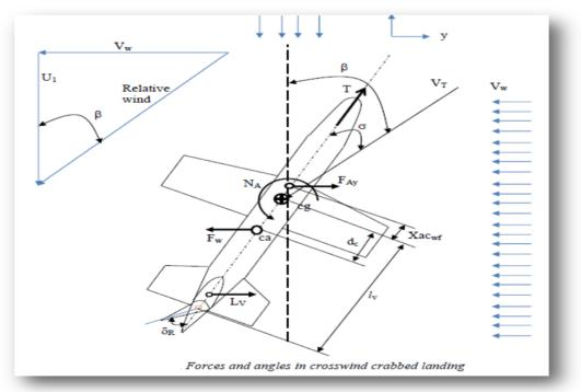
During the crosswind landing, rudder is applied to align the aircraft with the runway heading.
