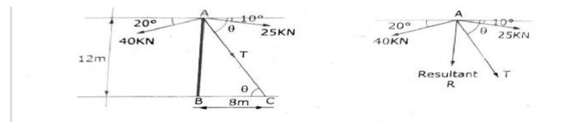
It is given that the resultant force is acting vertically downwards. Hence, the net horizontal force is zero (i.e.,  $\Sigma H = 0$ ) and the resultant force is equal to the net vertical force.
