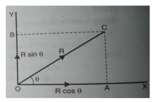
Components of R along x axis Components of R along y axis
