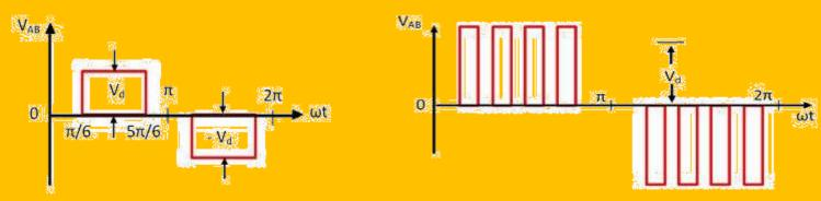
**Stepped wave & PWM wave output line voltage**
