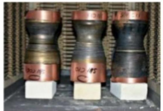
Liners were annealed to relieve residual stresses
