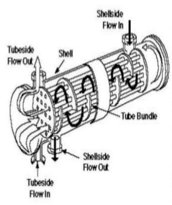
Gas turbine regenerators are usually constructed as shell-and-tube type heat exchangers using very small diameter tubes, with the high pressure air inside the tubes and low pressure exhaust gas in multiple passes outside the tubes
