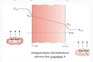
Boundary conditions:  $T(o) = T_{s,t}$  $T(L) = T_{s,2}$
