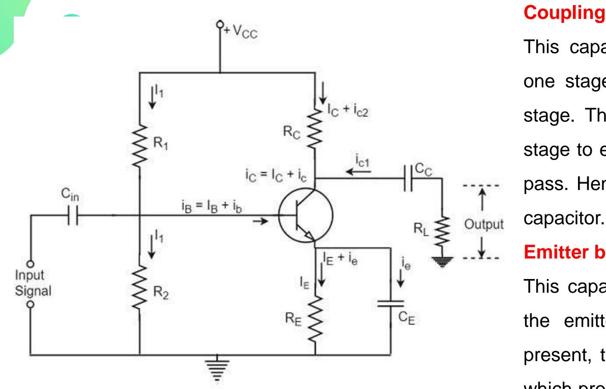
This capacitor is employed in parallel to the emitter resistor  $R_F$ . If this is not present, that signal will pass through  $R_{F}$ which produces a voltage drop across  $R_{F}$ will feedback the input signal 03/08 that **19EIB201/ED/Ms.B.Divya/AP/BME** radualar tha autout valtara
