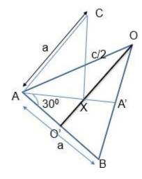
AB = AC = BO = 'a'. CX = c/2 where  $c \rightarrow$  height of the hcp unit cell.
