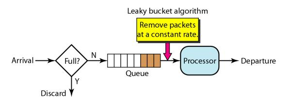
A leaky bucket algorithm shapes bursty traffic into fixed-rate traffic by averaging the data rate. It may drop the packets if the bucket is full.
