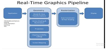
• Application – anything that the programmer wants. Interactions, loading of models, etc. Feed scene information into Geometry stage.
