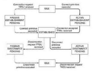
A state diagram for a simple connection management scheme. Transitions labeled in italics are caused by packet arrivals. The solid lines show the client's state sequence. The dashed lines show the server's state sequence.
