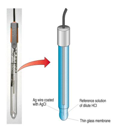
pH electrodes are able to determine the pH because they contain a solution of dilute HCl separated by a thin glass membrane from the test solution. The potential difference between the two different concentrations of H<sup>+</sup> is proportional to the pH.
