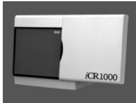
Figure 12.8 Tabletop-computed radiography cassette scanner. The screen is removed from the cassette, scanned, and returned to the cassette for the next exposure. The image information is sent to a computer for display and analysis. (Photo courtesy of iCRco.)
