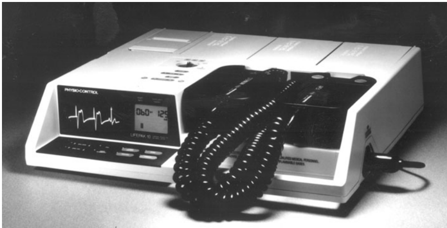
► Fig. 26.4 Portable external defibrillator, ECG monitor and recorder (Courtesy: M/s Physio Control, USA)
