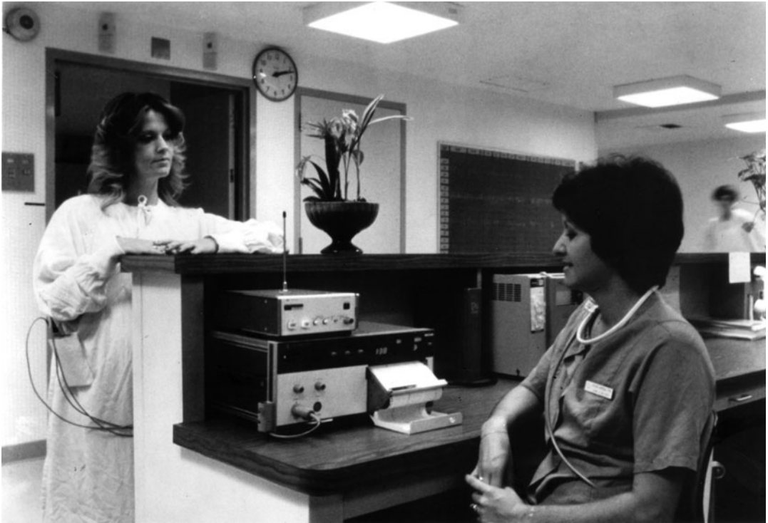
► Fig. 9.11 Telemetry receiving system for monitoring foetal heart rate and uterine contractions in use (Courtesy: Hewlett Packard, USA)
