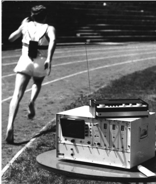
► Fig. 9.12 A three channel telemetry system to monitor the physiological data of a sprinter
