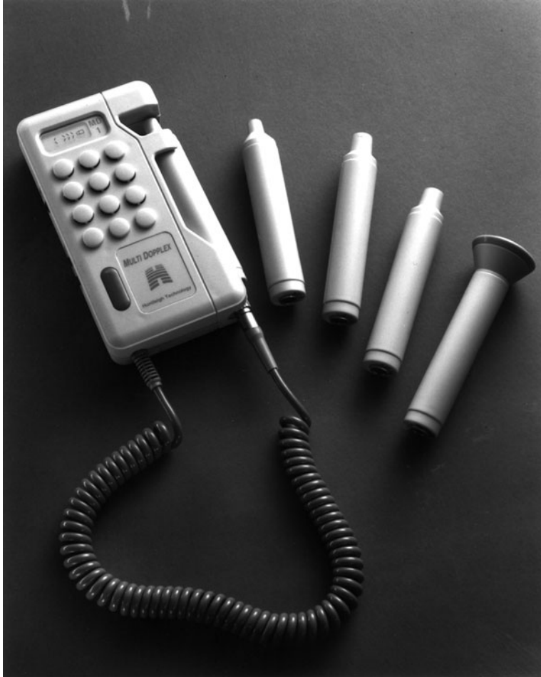
► Fig. 8.5(a) Ultrasonic blood flow detector (Courtesy: M/s Huntleigh Health Care, USA)
