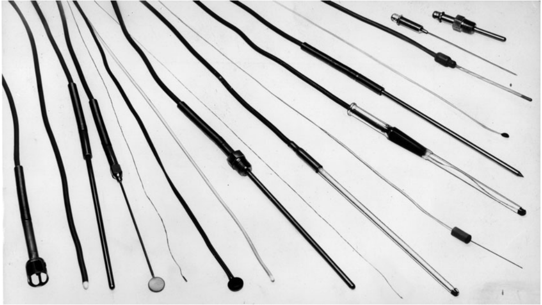
► Fig. 3.13 Different shapes of thermistor probes (Courtesy: Yellow Springs Instruments Co., USA)
