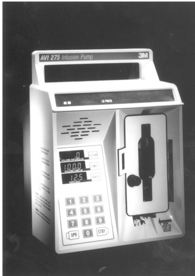
➤ Fig. 35.8 Programmable microprocessor based infusion pump (Courtesy: AVI, Inc. USA)
