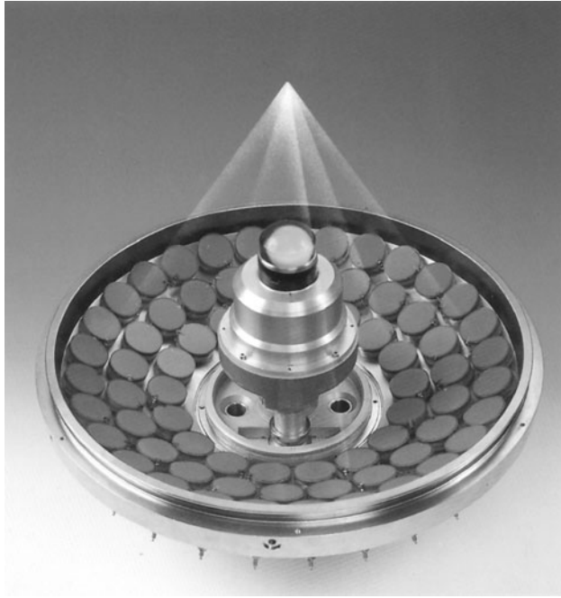
► Fig. 31.11 Inside view of lithotripsy treatment head using piezo-electric ceramic elements (Courtesy: EDAP International S.A., France)
