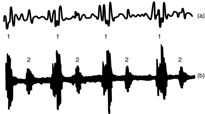
► Fig. 8.3 Foetal phonocardiogram: (a) unfiltered heart sounds, (b) filtered heart sounds
