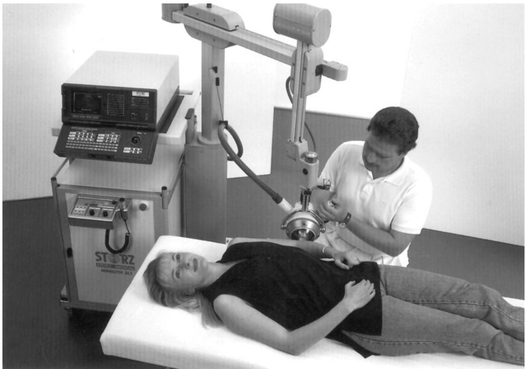
► Fig. 31.12 Shock-wave head with integrated ultrasound imaging. The sonographic probe is arranged centrally in the shock wave oscillation system. (Courtesy: M/s Storez Medical Co. Switzerland)
