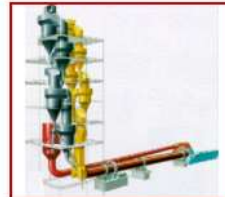
Preheater and Kiln
