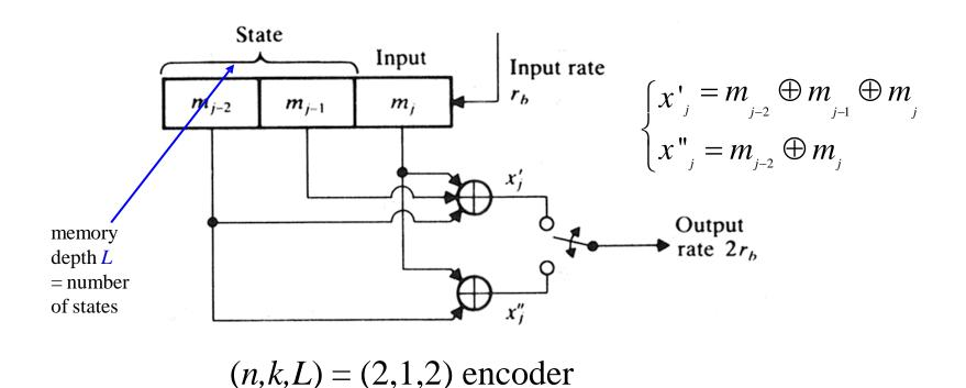
• Thus, for generation of n-bit output, we require in this example n shift registers in k = 1 convolutional encoder
