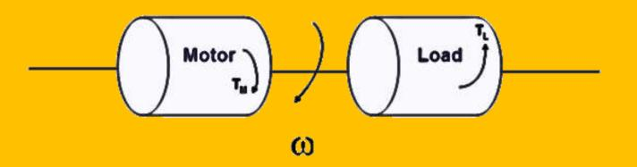
J = Moment of inertia of motor load system referred to the motor shaft kg / sq.m
