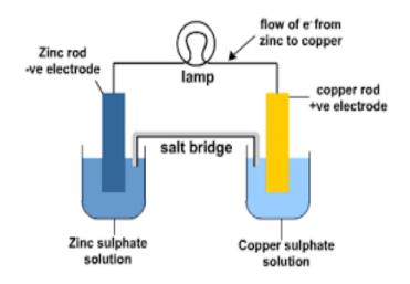
It consists of a zinc electrode dipped in 1 M zinc sulphate solution and a copper electrode dipped in 1 M copper sulphate solution. Each electrode is considered as a half cell. The two standard half cells are coupled by salt bridge and to form a cell. The electrode reactions are as follows: **At anode :** Zinc passes into solution as zinc ion and liberates two electrons at the electrode. Here, oxidation reaction occurs at the zinc electrode.
