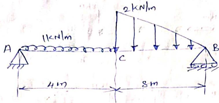
Converting UDL into point Load.
