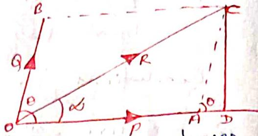
It states that "if two forces act simultaneously at a point be represented magnitude & direction, by the two adjacent sides of a parallelogram, then the resultant of these two forces is represented in magnitude and direction by the diagonal of that parallelogram originating from the point."
