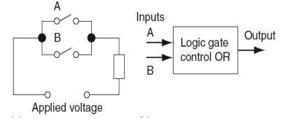
Figure (a)Truth table of the OR logic (b) block diagram of OR logic
