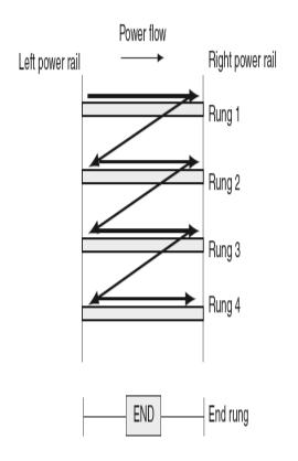
1. The vertical lines of the diagram represent the power rails between which circuits are connected. The power flow is taken to be from the left-hand vertical across a rung.
