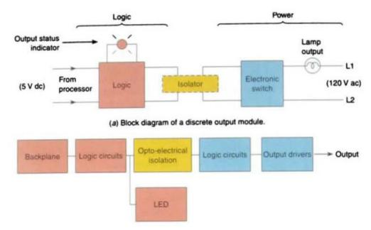
Discrete output modules are used to turn real world output devices either on or off.
