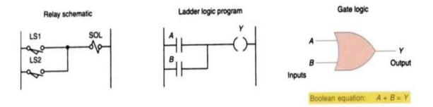
• Two limit switches connected in parallel and used to control a solenoid valve.
