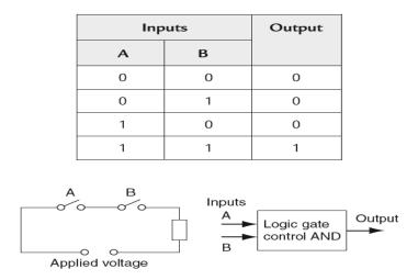
Figure (a)Truth table of the AND logic (b) block diagram of AND logic
