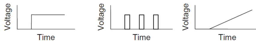
Fig 3. Types of signals: Discrete, Digital and Analog.
