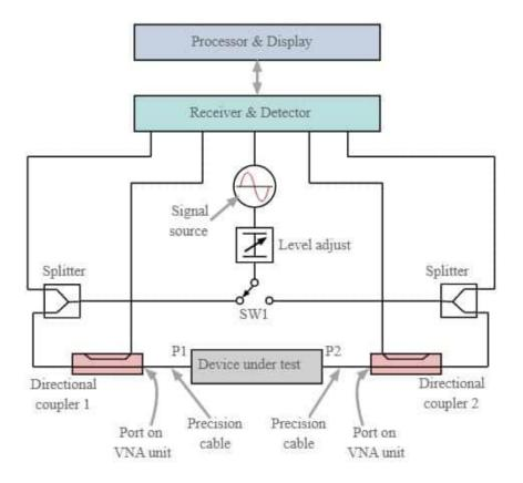
Radio frequency (RF) network analyzers are test and measurement instruments used to characterize the performance of RF and microwave components and systems. RF network analyzers can measure insertion loss, return loss, and S-parameters of RF and microwave devices and systems.
