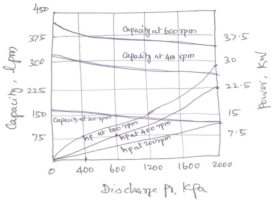
The curve showing the relationship between Pump discharge pressure and pump capacity is head - capacity or HQ curve.
