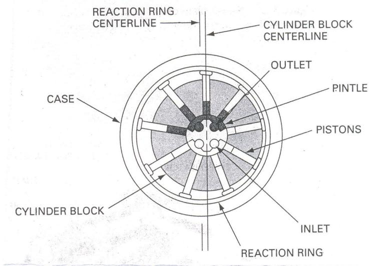
As cylinder barrel rotates, the pistons on one side travel outward. This draws in fluid as each cylinder passes the suction ports of the pintle. When a piston passes the point of maximum eccentricity, it is forced inward by the reaction ring. This forces the fluid to enter the discharge port of the pintle.
