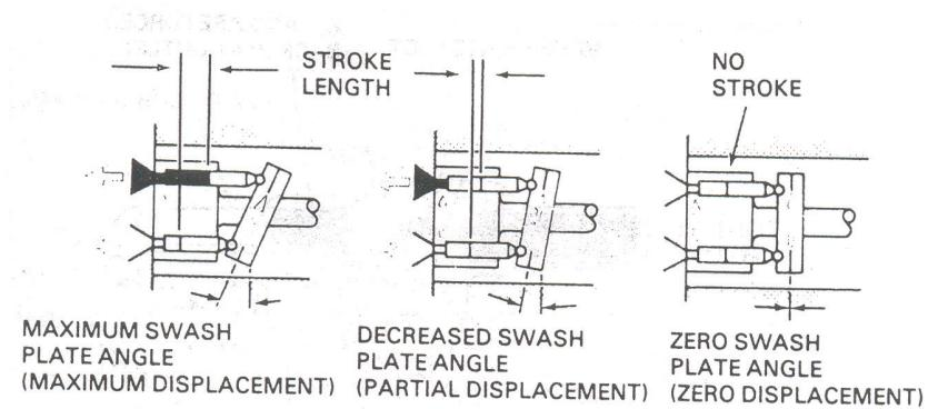
As the cylinder rotates, the pistons reciprocate because the piston shoes follow the angled surface of swash plate. The inlet and outlet ports are located in the valve plate so that the pistons pass the inlet as they are being pulled out and pass the outlet as they are being forced back in.
