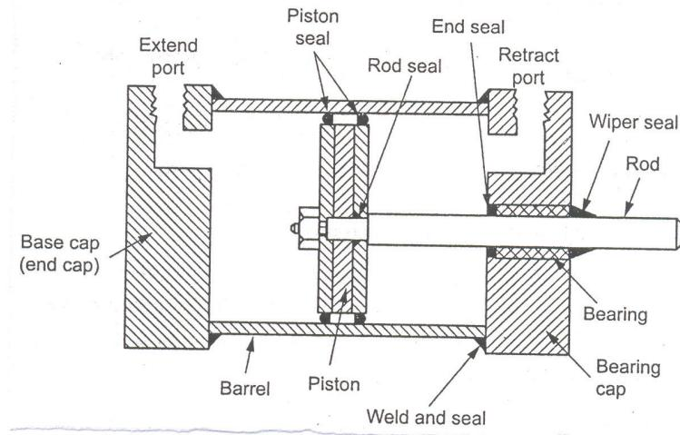
The Components are designed in such a way that the end caps and pistons are common to all cylinders of the same diameter and only barrels and piston rod need to be changed to construct different length cylinders. The end caps are welded to the barrel and the piston rods are threaded to the piston.
