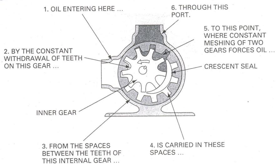
a regular spur gear, a crescent-shaped seal, and an external housing. The crescent seal placed acts to ensure a seal between suction and discharge.
