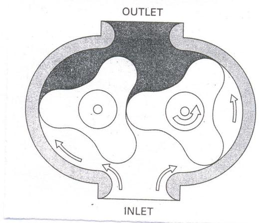
Thus, they are quieter than the other types of gear pumps. Due to smaller number of mating elements, the lobe pump output will have somewhat greater amount of pulsation, although its volumetric displacement is generally greater than that for other types of gear pumps.
