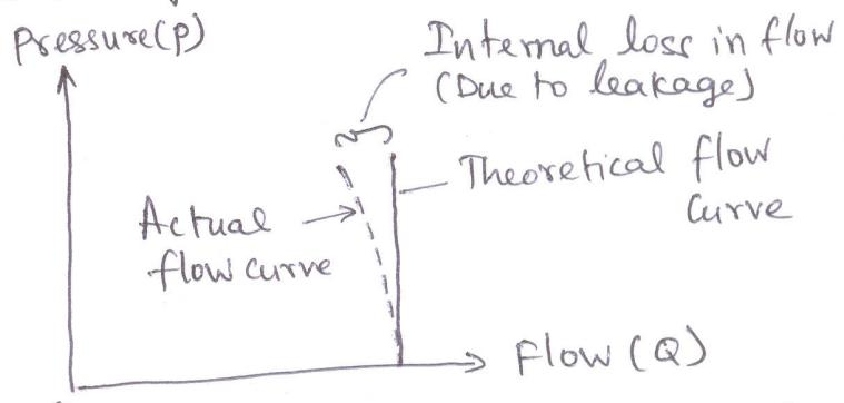
If Pressure increases, internal flow loss increases.
