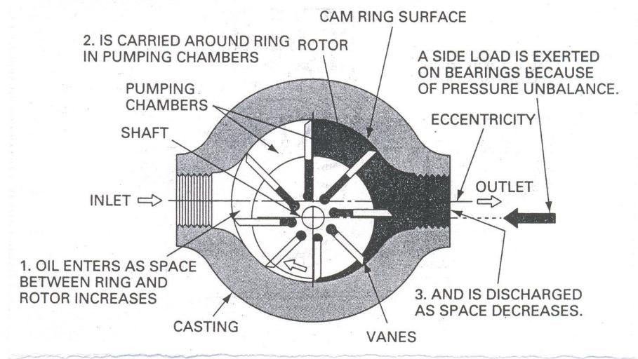
The eccentricity between the centre of the rotor and Cam ring is responsible for making the flow rate. As the eccentricity can be varied, this Vane pump may be called as Variable displacement pump. If the eccentricity is zero there will be no flow, the flow is maximum when the eccentricity is maximum.
