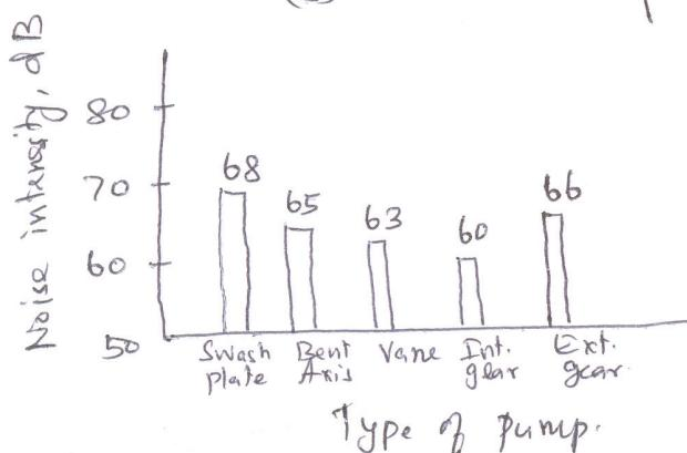
Any pump which generates noise above 70 dB(A) is loud pump. Those around 60 dB(A) or less are considered quiet running.
