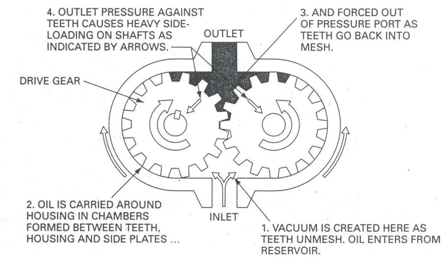
When the pump starts, in suction side where teeth come out of mesh, volume expands and pressure reduces below atmosphere i.e. partial vacuum. So the fluid from reservoir is forced into the pump inlet. In the discharge side, teeth go into mesh and the volume decreases between the mating
