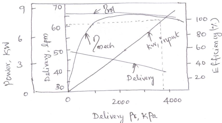
This graph shows how much power must be supplied to the pump to obtain different rates of discharge against different discharge pressures.
