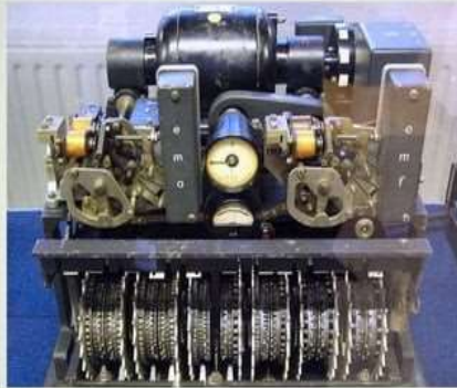
German Lorenz cipher machine, used in World War II to encrypt very-high-level general staff messages.
