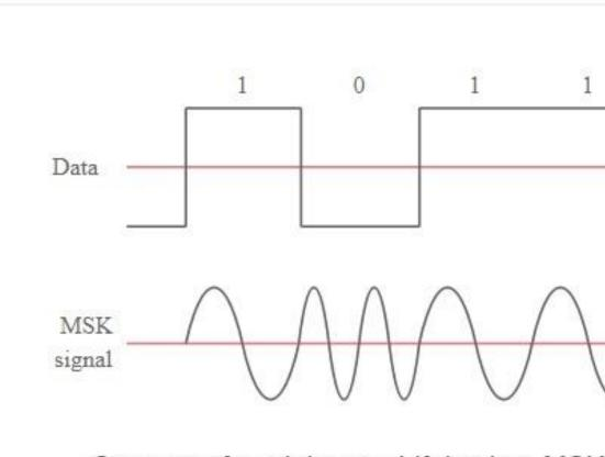
Concept of a minimum shift keying, MSK signal
