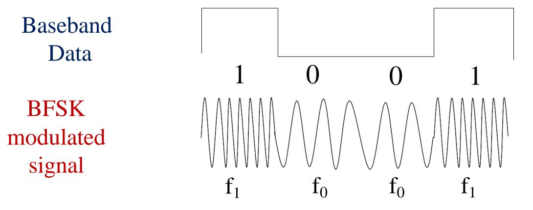
where  $f_0 = A\cos(\omega_c - \Delta\omega)t$  and  $f_1 = A\cos(\omega_c + \Delta\omega)t$
