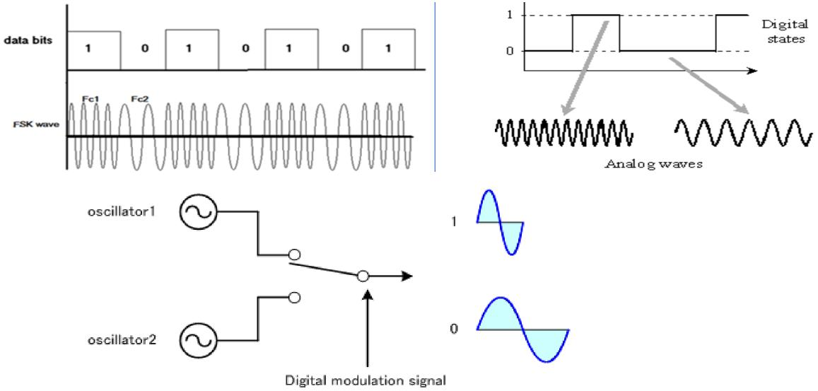
Switch between two oscillators accordingly
