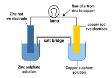
It consists of a zinc electrode dipped in 1 M zinc sulphate solution and a copper electrode dipped in 1 M copper sulphate solution. Each electrode is considered as a half cell. The two standard half cells are coupled by salt bridge and to form a cell. The electrode reactions are as follows:
