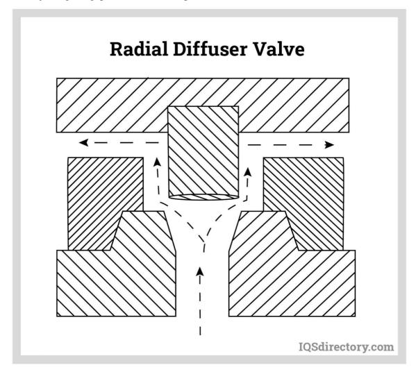
In this type of homogenizer valve, the premix fluid initially flows axially and is deflected at a  $90^{\circ}$  angle by the plug. This forces the fluid to flow radially along the small gap. After exiting the gap, the fluid stream hits an annular surface called an impact or wear ring.
