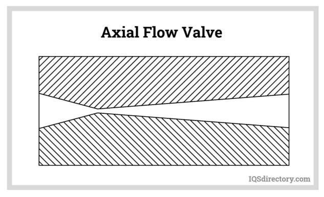
The premix remains flowing axially as it passes through the orifice. Shearing, cavitation, and turbulence also take place within the small gap. Upon exiting the gap, the fluid jet is expanded without an impact chamber, unlike what is seen in a radial diffuser valve.
