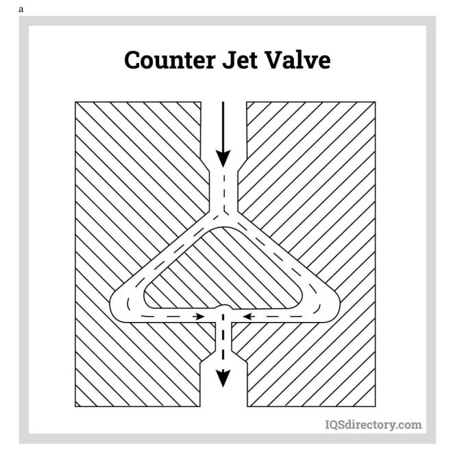
The benefit of using a counter jet valve is the operation without moving parts. Thus, they have greater reliability than radial diffuser valves. Moreover, no impact ring tends to wear over time due to the continuous impingement of the fluid.
