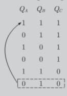
For the state 010 all preset = 1 and output  $Q_A Q_B Q_C = 111$  so here total no. of states = 5 (down counter)
