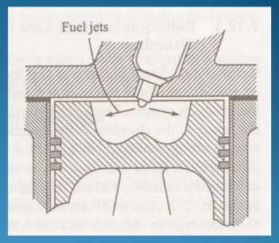
Figure shows a bowl-in-piston type of medium swirl open chamber with a centrally located multihole injector nozzle. The amount of liquid fuel which impinges on the piston cup walls is kept minimum. This type is used in medium size (10 to 15 cm bore) diesel engines.
