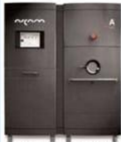
ARCAM A2 machine for direct metal deposition
