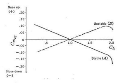
The slope of this curve of  $C_m$  versus  $C_L$  is given by the derivative  $dC_m/dC_L$ , and a negative sign for this derivative is required for static longitudinal stability. The slope of the pitching moment curve  $dC_m/dC_L$  can be obtained analytically by differentiating equation (5-4) with respect to  $C_L$ :
