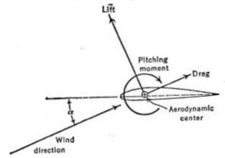
K.NEHRU, M.Tech., (Ph.D). Assistant Professor The lift and drag are by definition always perpendicular and parallel to the wind, respectively. It is therefore inconvenient to use these forces to obtain moments, for their arms to the center of gravity vary with angle of attack. For this reason all forces are resolved into normal and chordwise forces whose axes remain fixed with the airplane and whose arms are therefore constant.
