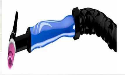
Water-cooled TIG torches have a gas input while having an input and output for water lines. This is an advantage for **larger projects** that need rapid cooling. This comes with its price though, as a water cooler system has to be installed.
