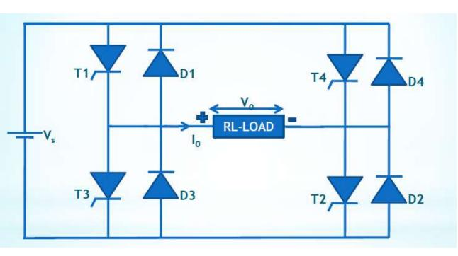
**MODE 1**: T1, T2 ON, SOURCE DELIVERING POWER TO LOAD – Vo +ve, lo +ve.
