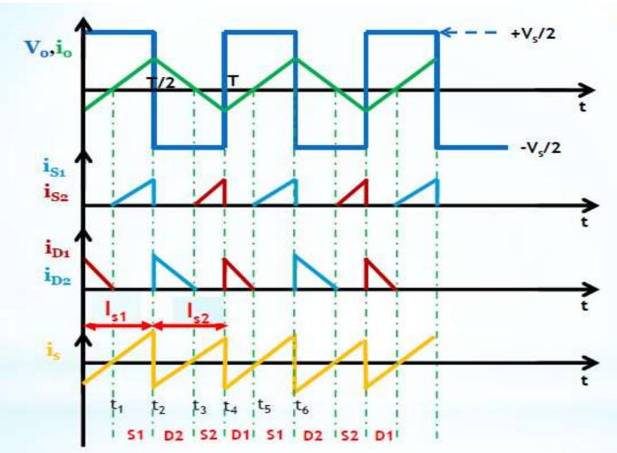
$$V_o(rms) = \frac{1}{T_0/2} \int_0^{T_0/2} \frac{V_s^2}{4} dt = \frac{V_s}{2}$$
