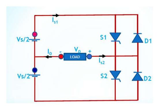
Mode1: S1-ON, Vo is +ve, Io is +ve, Is1 is +ve. Load takes power from source; VT2=Vs, VD1=0V, VD2= -Vs.
