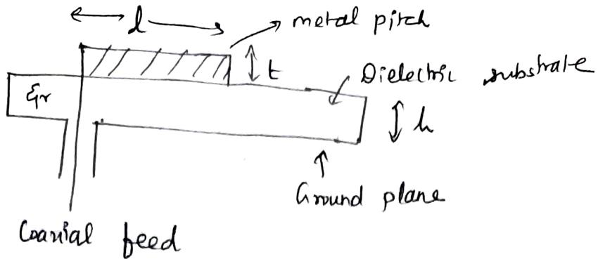
\* The Patch Antenna acts as a resonant  $\lambda/2$  Parallel plate microstrip transmission line with chara impedance equal to the reciprocal of the no of parallel field cell transmission lines
