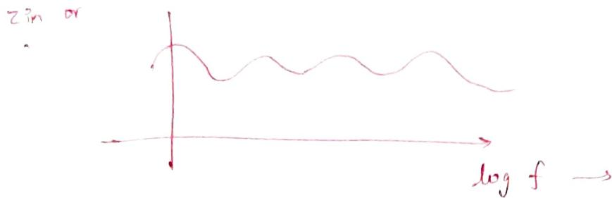
\* The ilp impedance is a logarithmically periodic function of frequency. Not only this, all the electrical properties undergo similar periodic variation particularly radiation pattern, directive gain, side lobe level, beam width and beam direction.
