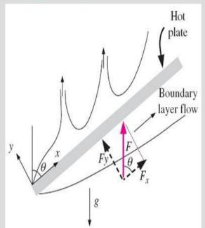
Natural convection flows on the upper and lower surfaces of an inclined hot plate.
