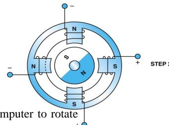
Most stepper motors use four wires, which are pulsed by the computer to rotate the armature in steps.
