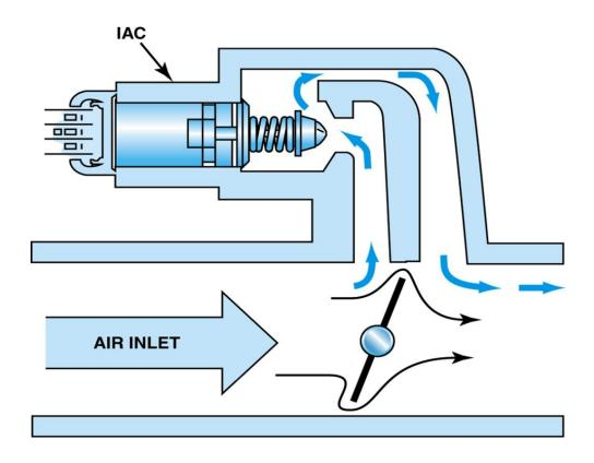
The small arrows indicate the air bypassing the throttle plate in the closed throttle position. This air is called minimum air. The air flowing through the IAC is the airflow that determines the idle speed.
