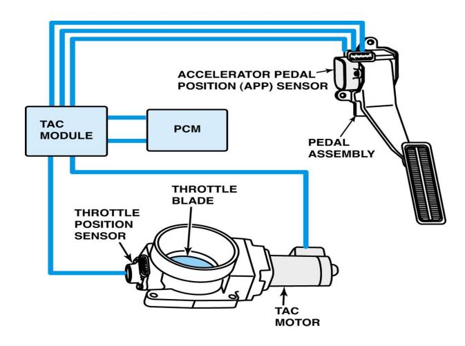
A GM electronic throttle control system showing the APP and TP sensors and the DC throttle actuator control (TAC) module and PCM. In many systems the motor control is located inside the PCM.
