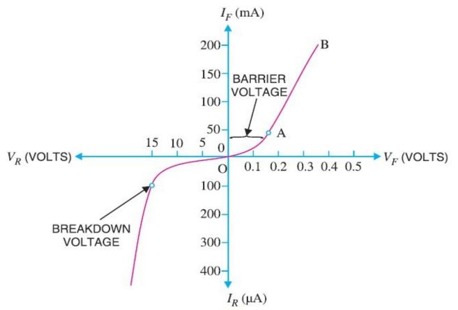
The curve drawn between voltage across the junction along x axis and current through the y axis.
