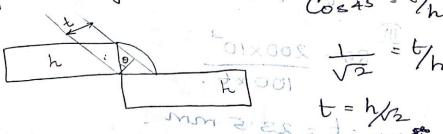
Peoblems o 1 Two plates soined by fillet weld and are subjected to tensile force of 200 kN if allowable show steers of weld is 85 MPas. Calculate the size of the weld 9 Soln: L= 125 mm. 100 mm. Double Parallel fillet weld! food & weld shed 103 = 288 (100+(2×125))+ blow tillet when t = 6.72mm h = 9.5 mm. 85 = 200 × 103 (2x125) t
