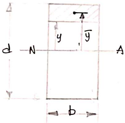
We want to find the bending shear stress  $\tau$  at a distance  $y$  from the neutral axis.
