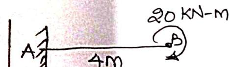
$$\begin{aligned} \text{Bending moment} \\ \text{at A} &= 20 \text{ KN-m} \\ &\text{only.} \end{aligned}$$
