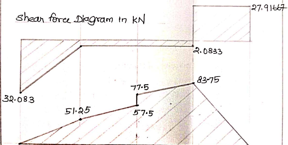
Bending Moment Diagram in kN-m.
