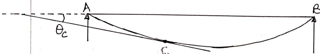
Consider a cantilever beam and a simply supported beam. Slope at the point C in both beams are to be found. To do so, draw a tangent at the point C to the deflection curve. Extend the tangent to meet the undeflected beam position. The angle between the tangent and the original beam is the slope at point C.
