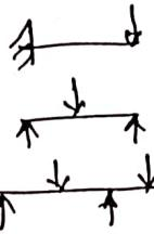
Indeterminate Beams : Propped cantilever beam
