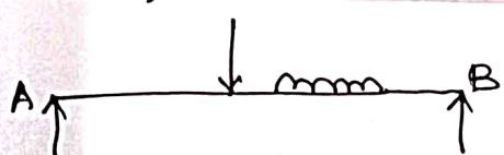
$R_A, R_B$  = Support reaction forces at A & B respectively.
