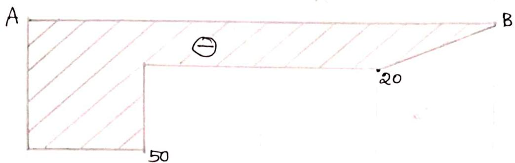
Bending Moment Diagram in kN-m
