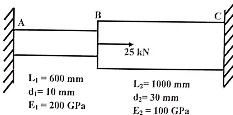
From the loading diagram, we can infer that region AB undergoes tension, i.e., region AB elongates and region BC undergoes compression, i.e., region BC shortens. Also we can infer that some portion of the total load is used to elongate region AB and the remaining portion of the total load is used to shorten region BC.
