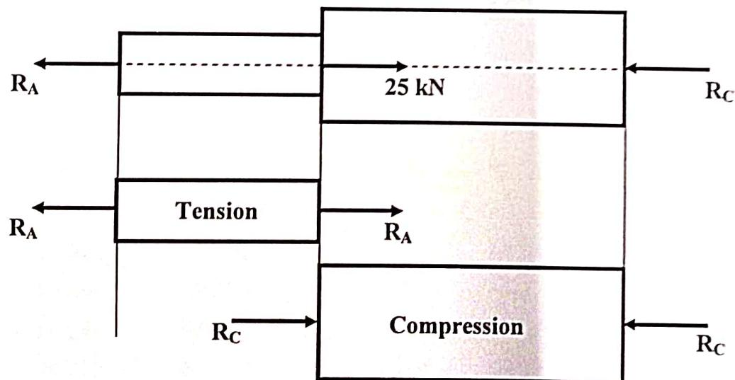
Equation (1) cannot be solved since there are two unknowns. Hence, the given stepped bar is an indeterminate bar. To solve this indeterminate bar, we need “compatibility” equation or “compatibility” condition which is given by
