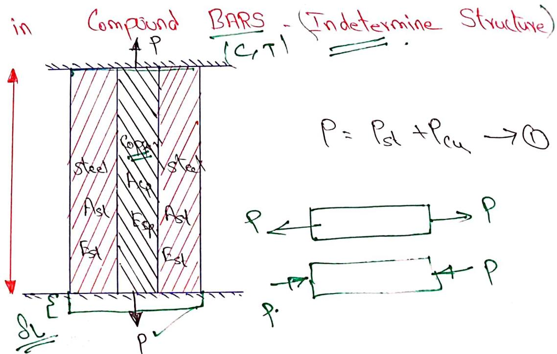
$\therefore$  Elongation of Steel Bar = Elongation of Copper Bar
