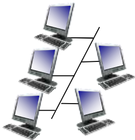
shared wire (e.g., cabled Ethernet)
