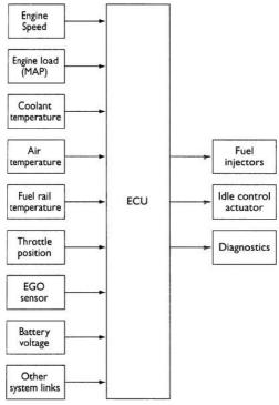
Figure 18. Block diagram of inputs and outputs common to most fuel injection systems
