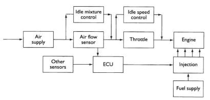
Figure 17. Typical control layout for a fuel injection system
