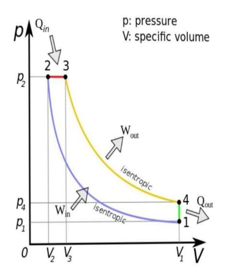
PV diagram for the ideal diesel cycle (which follows the numbers 1-4 in clockwise direction). The horizontal axis is the cylinder volume. In the diesel cycle the combustion occurs at almost constant pressure. On this diagram the work that is generated for each cycle corresponds to the area within the loop.
