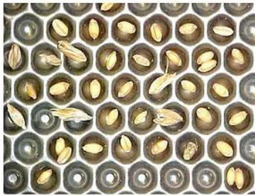
Interior of Indented Cylinder
