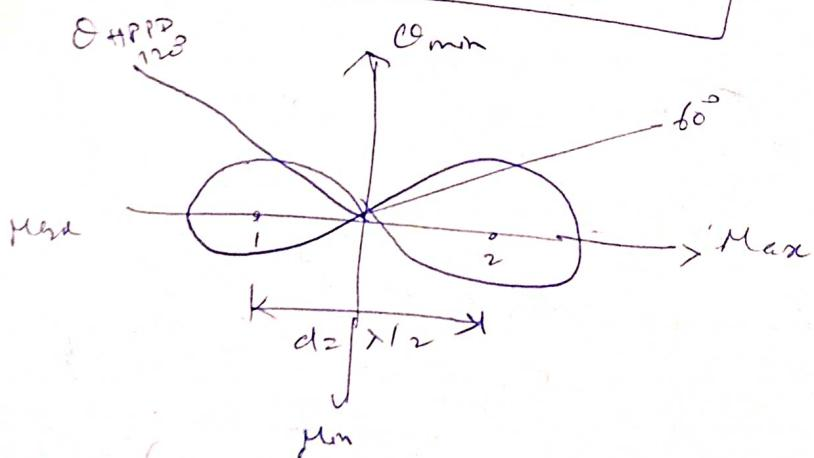
Field Pattern of two isotropic point sources of same amplitude but opposite phase spaced  $\lambda/2$  apart
