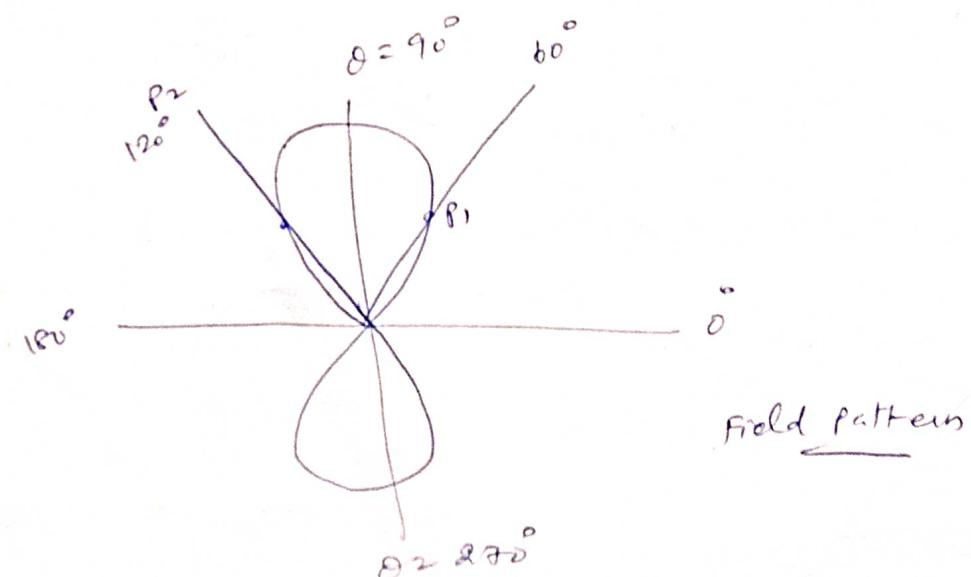
(ii) Array of two point sources of unequal amplitude and any phase
