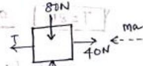
D'Alembert's principle states the body is in equilibrium condition, with the imaginary force 'ma' (called inertia force) in opposite direction.
